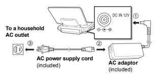
The unit is in the standby condition (the [ $\circlearrowleft$ ] indicator lights) when the AC power supply cord is connected. The primary circuit is always "live" as long as the AC adaptor is connected to an electrical outlet.
